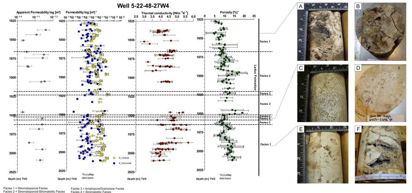
Fig. 2: Measurement results of apparent permeability and thermal conductivity from well 5-22-48-27W4 of the Leduc Formation in correlation with permeability and porosity measurements from the AccuMap data base. Facies were defined according to shape and size of the vugs and molds of the dissolved parts, classified by Drivet (1993). Exemplary core samples are shown on the right (depth: A and B = 1843.1 m; C and D = 1957 m and E and F = 1993.4 m).
