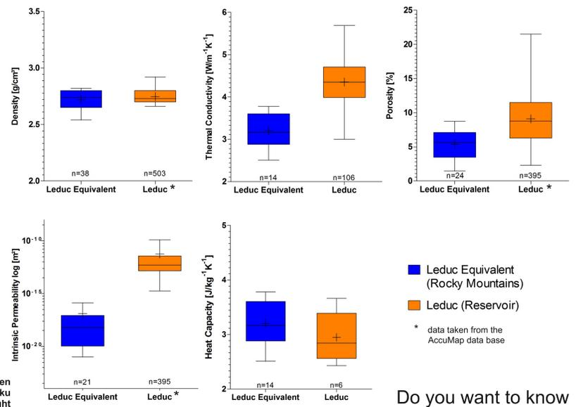
Fig. 4: Comparison of exemplary average rock properties of the Leduc Formation and the Leduc Equivalent in the Rocky Mountains.
