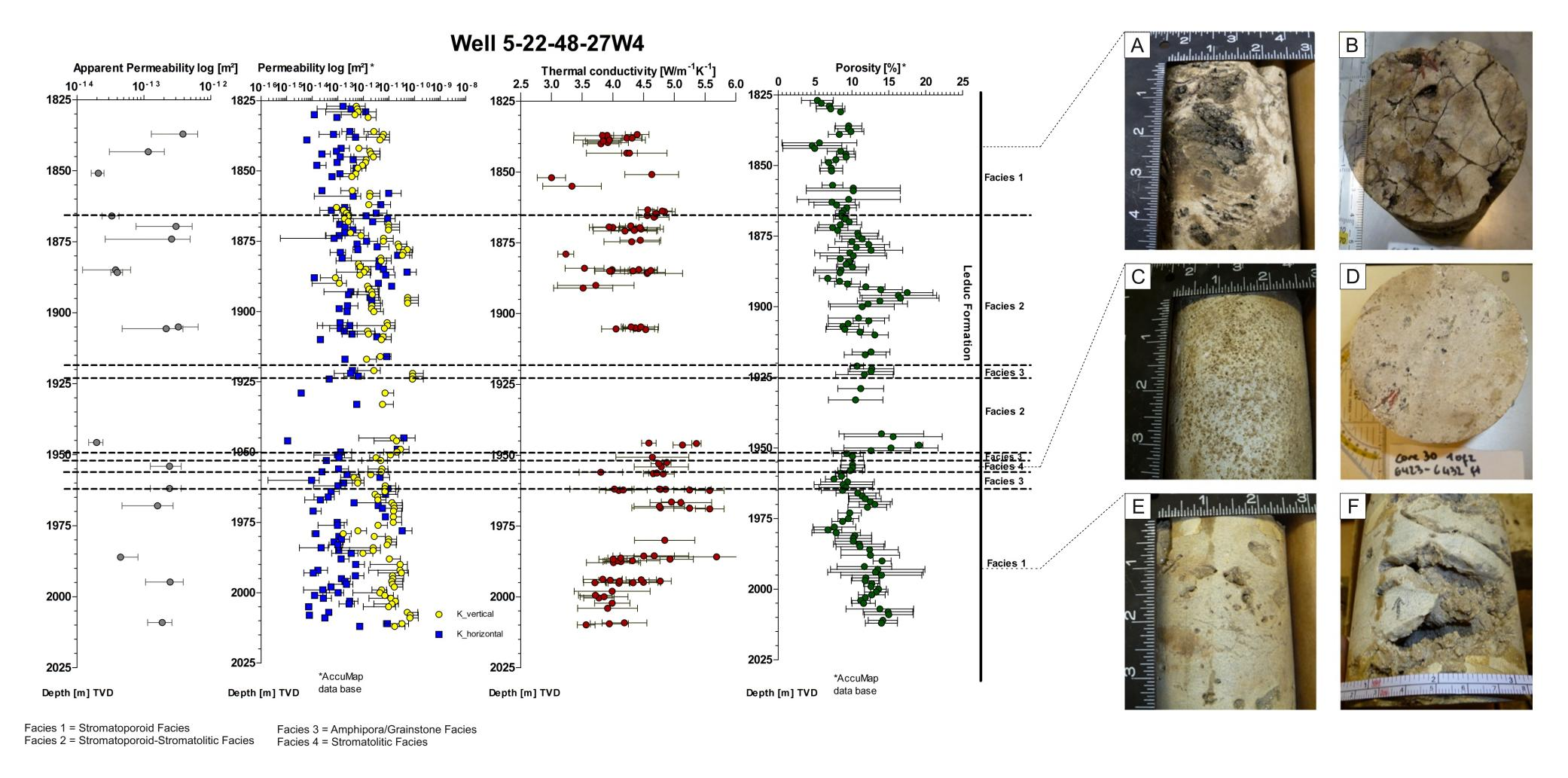
To accomplish the analogue study acquiring geothermal and petrophysical rock properties, samples from 3 analogue outcrops and 5 cores of the target reservoir were used. Parameters like density, porosity, permeability, thermal conductivity, thermal diffusivity, heat capacity as well as wave velocities were measured on the analogue samples at the TU Darmstadt laboratory (Darmstadt).
