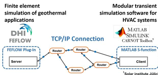
Figure 1: Coupling concept for the simulations of the subsystems.
