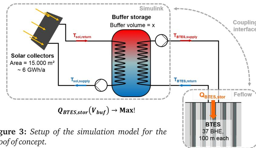
Figure 3: Setup of the simulation model for the proof of concept.
