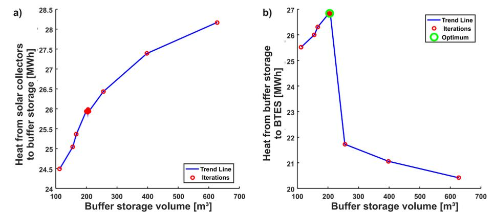
Figure 5: Heat amounts that are transferred (a) from the solar collectors to the buffer storage and (b) from the buffer storage to the BTES for the respective iteration of the buffer volume..
