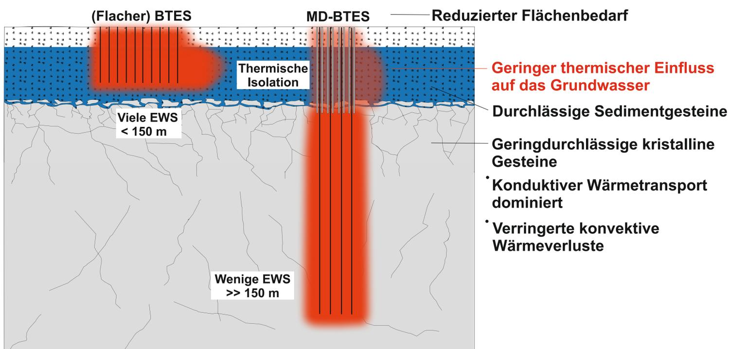
Verändert nach Seib L., Welsch B., Bossennec C., Frey M., Sass I. (2022): Finite element simulation of permeable fault influence on a medium deep borehole thermal energy storage system. Geothermal Energy, 10 (15)
